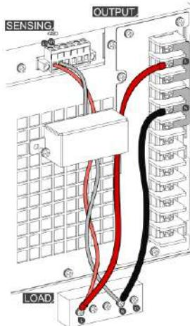
The remote sense connection and the protective lid installation are completed accordingly.
