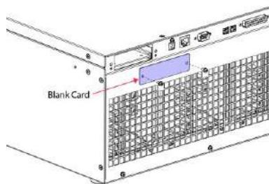
4. Insert an optional interface card (DeviceNet, CAN BUS, GPIB) into the slot of rear panel and click it all the way into place.
