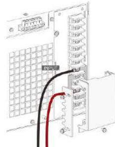
The AC power cords of Single phase input are connected with the AC input terminals equipped with protective lid completely.
