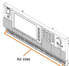
Follow the steps 1-3 in reversed order to reassemble the lid and the cover of air inlet with ASR-6000 unit.
