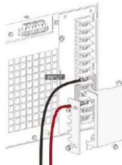
The AC power cords of Single phase input are connected with the AC input terminals equipped with protective lid completely.
