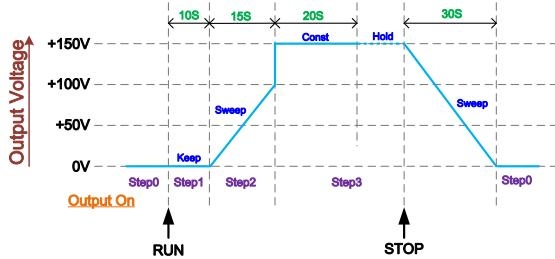
The example above shows how to generate a test procedure in DC-INT mode by each step.
