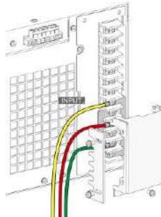
The AC power cords of Delta input are connected with the AC input terminals equipped with protective lid completely.
