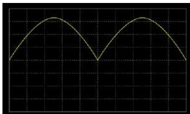
ARB 8 Sine wave, full-wave rectification (negative polarity)
