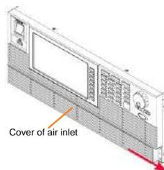
Remove the cover of air inlet via pulling it out of ASR-6000 unit outward.
