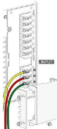
The AC power cords of NEW input are connected with the AC input terminals equipped with protective lid completely.
