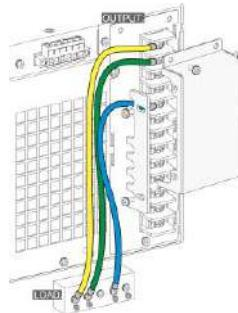
The AC power cords of 1P3W output are connected with the AC output terminals equipped with protective lid completely.
