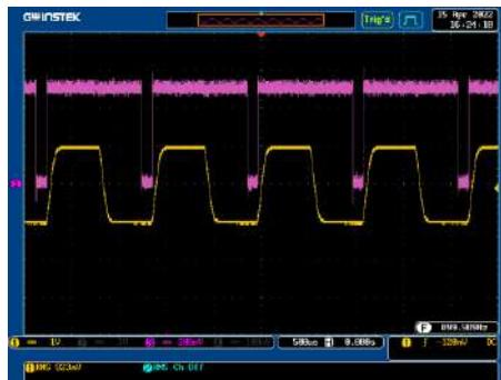
The actual waveform – AC-INT Mode, Frequency 900 Hz, TrgOut Width 1.1 ms
