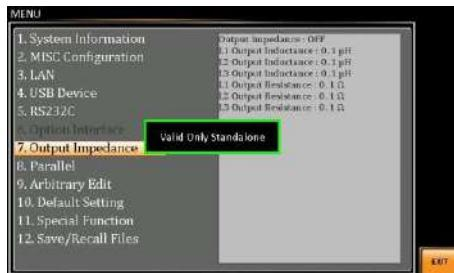
If there is any fluctuation in the output voltage when this function is initiated in conjunction with the DUT, the utilization of this function becomes impracticable.
