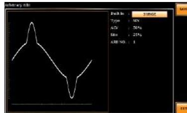
**DST01-30** The DST01-30 waveform shape function simply adds a number Fourier series terms to create an arbitrary waveform.
