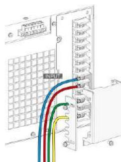
The AC power cords of Y input are connected with the AC input terminals equipped with protective lid completely.
