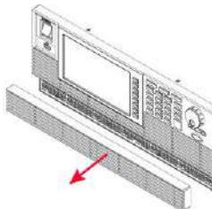
Use a vacuum cleaner to absorb and remove dust off from the air inlet.
