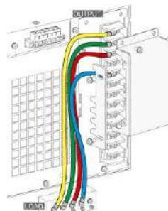
The AC power cords of 3P4W output are connected with the AC output terminals equipped with protective lid completely.
