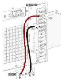
The AC power cords of 1P2W output are connected with the AC output terminals equipped with protective lid completely.
