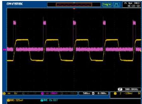
The actual waveform – AC-INT Mode, Frequency 900 Hz, TrgOut Width 1 ms
