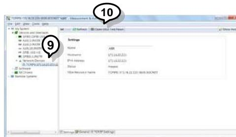
11. Click the *Configuration* Icon. Under the *IO Settings* tab check *Enable Termination Character*. The termination character should be set as *Line Feed - \n*.
