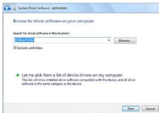
ASR-6000 will now be located in the *Ports* node of the hardware tree in the Windows Device Manager if the driver installation was successful.
