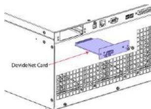
5. Fasten the screws to fix the optional interface card onto the rear panel of unit. The screws number varies per different interface card.
