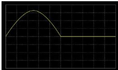
ARB 6 Sine wave, half-wave rectification (negative polarity)
